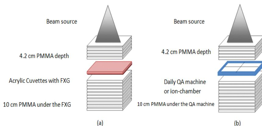
**Fig. 2. Setup with PMMA phantom for open and wedged X-ray beam profiles, open electron beam profiles and X-ray output factor with 4 plates  $30 \times 30 \times 1 \text{ cm}^3$  and one plate  $30 \times 30 \times 0.2 \text{ cm}^3$  up and 10 plates  $30 \times 30 \times 1 \text{ cm}^3$  down to the examined FXG samples (a) or daily QA machine (b).**
