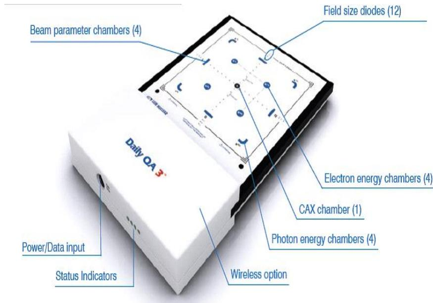
**Fig. 1. The SUNNUCLEAR Daily QA<sup>TM</sup> instrument.**
