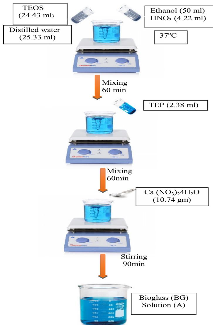
**Fig.1. Flowchart for Bioglass preparation steps.**
