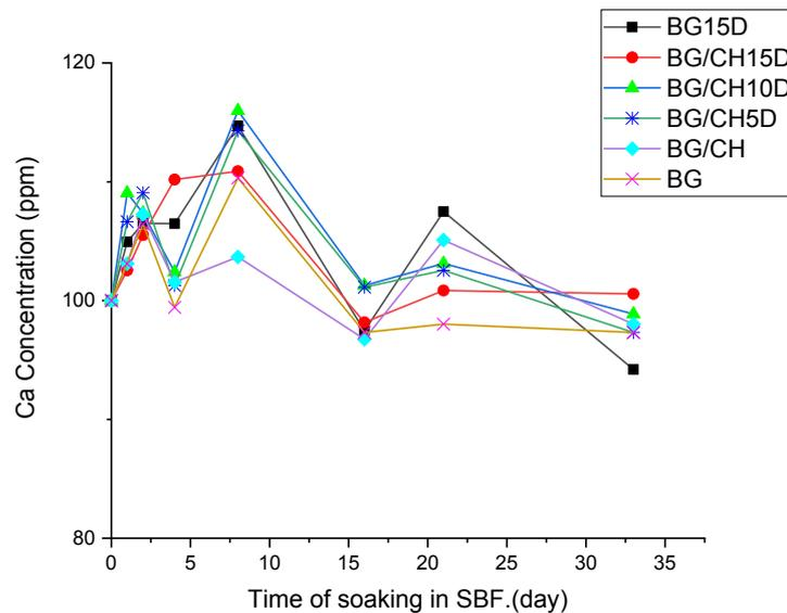
Fig. 10. The concentration of  $\text{Ca}^{2+}$  ions after soaking in SBF solution for 33 days.
