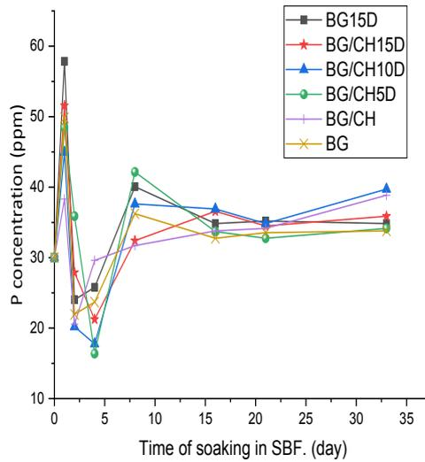
Fig. 11. The concentration of P<sup>5+</sup> ions in SBF solution after soaking for 33 days.
