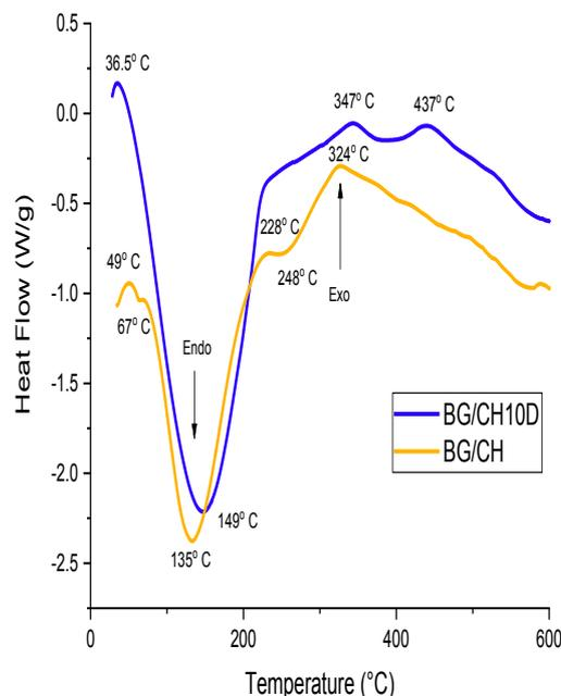
Fig. 5. DSC thermo analysis curves of BG/CH and BG/CH10D samples.
