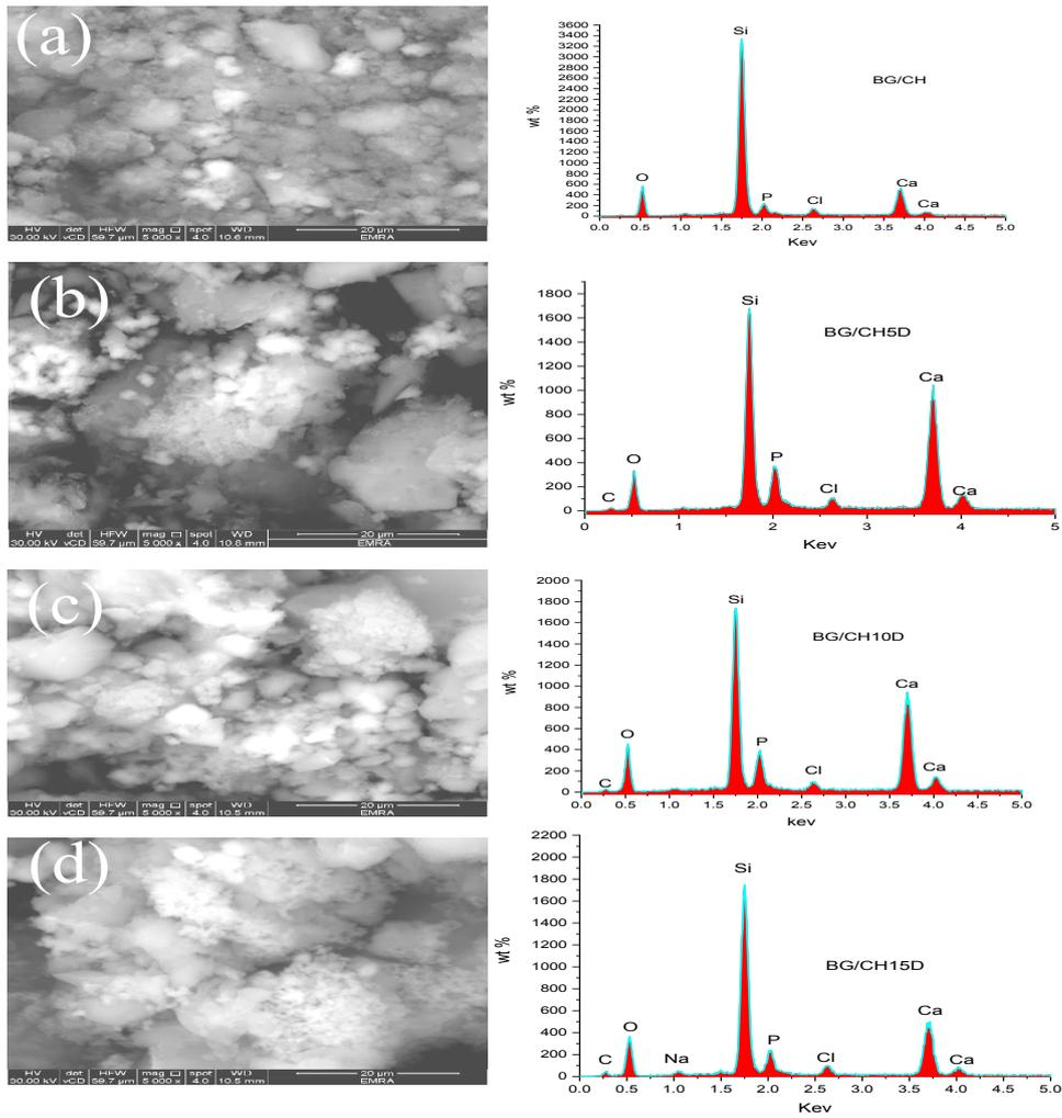
Fig. 8. SEM image – EDX spectrum of (a) BG/CH (b) BG/CH5 (c) BG/CH10D (d) BG/CH15D after immersion in SBF for 33 days.
