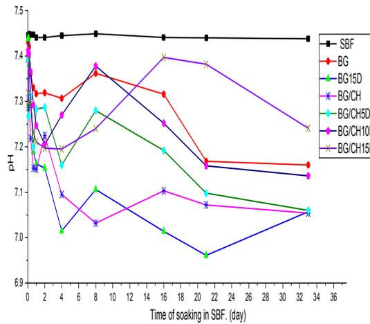
Fig. 12. The change in pH results of BG, BG/CH and BG/CH loaded with Dexamethasone after immersion in SBF for 33days.
