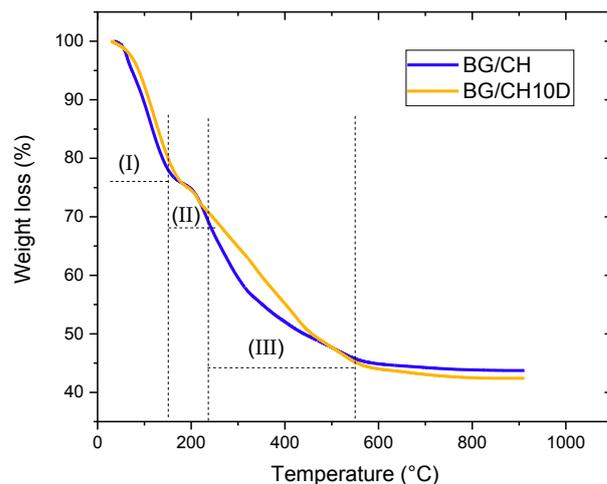
Fig. 4. TGA curves of BG/CH and BG/CH10D samples.
