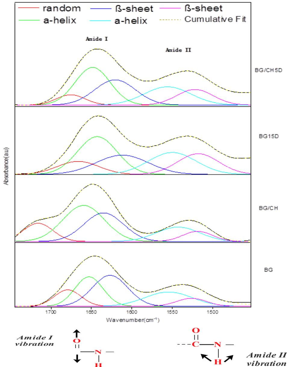
Fig. 6. FTIR spectra of the Amide I and Amide II bands of BSA adsorbed on the surfaces of the samples.
