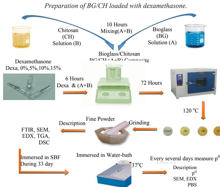
Fig.3. Flowchart for preparation of the BG/CH composite with dexamethasone loaded and investigate steps.
