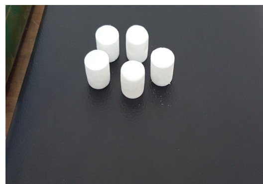
Fig. 1. The freeze-dried spongy structure scaffold samples of cylindrical forms.
