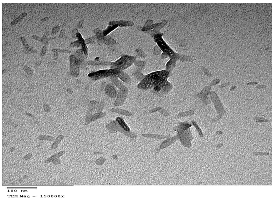
**Fig. 3. TEM image of ZnO nanoparticles.**
