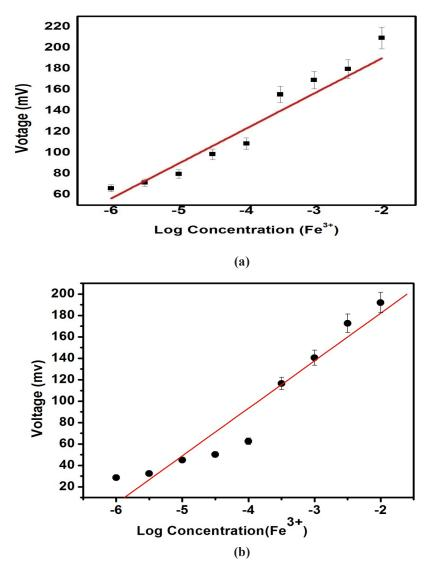
Fig.3(a&b).The calibration curve of the log concentration for Fe<sup>3+</sup>ionsin FeCl<sub>3</sub> solution as a function of electrochemical potential difference by using ZnO-(NRs)TF deposited on(a)conducting Plastic substrate (b) silicon substrate, for bio-sensor application.
