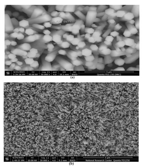
Fig.2 (a&b). FESEM images of ZnO-(NRs)TF grown on (a) plastic substrateannealed at 150°C (b) siliconsubstrates annealed at 250°C, for biosensor application.
