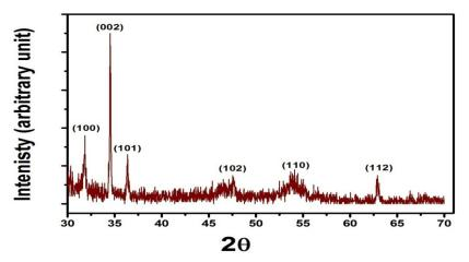
Fig. 1.x-Ray Diffraction of ZnO-(NRs)TF deposited on plastic substrate.
