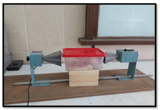
Fig.1. Microwave exposure system.
