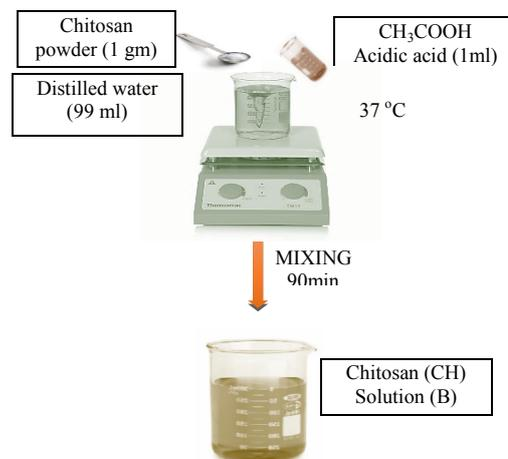
Fig.2. Flowchart for Chitosan preparation steps.
